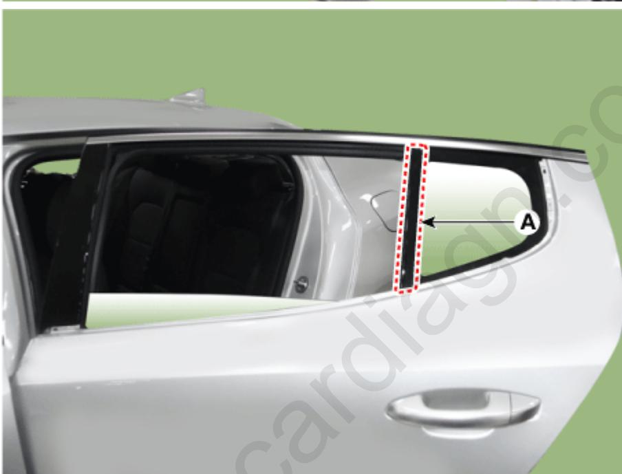
6. Remove the rear door frame molding (A) by using a remover.
